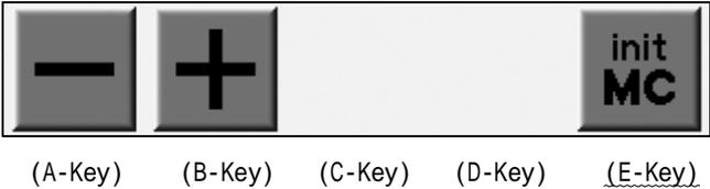
3) Press the A-Key to initialize the MC Parameters.
