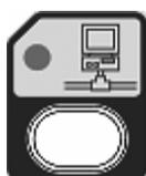
The blinking LED on the Network Key shows that the Network has been made.
