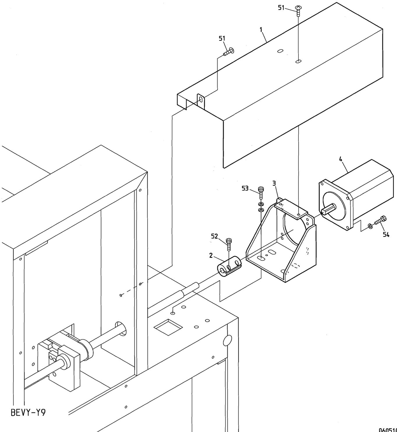
10G-2 Pantograph drive G (Medium pulse motor)
